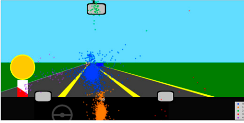
Figure 4. Clustering of fixations shown on example participant (Participant 5). Clusters 0, 1, 2, 4 can be assigned to specific locations (upcoming road, speedometer, rear-view mirror, and left lane, respectively). Cluster no. 3 cannot be assigned to a location and accounts for noise.
